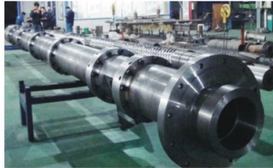
XPS-300二氧化氮发泡螺杆机筒 Φ300 XPS Nitrogen dioxide foam screw and barrel
