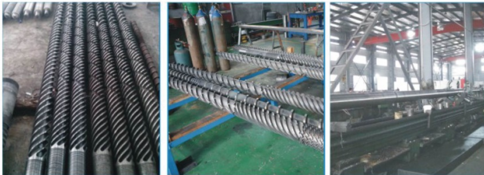
XPS-300二氧化氮发泡螺杆机筒 Φ300 XPS Nitrogen dioxide foam screw and barrel
