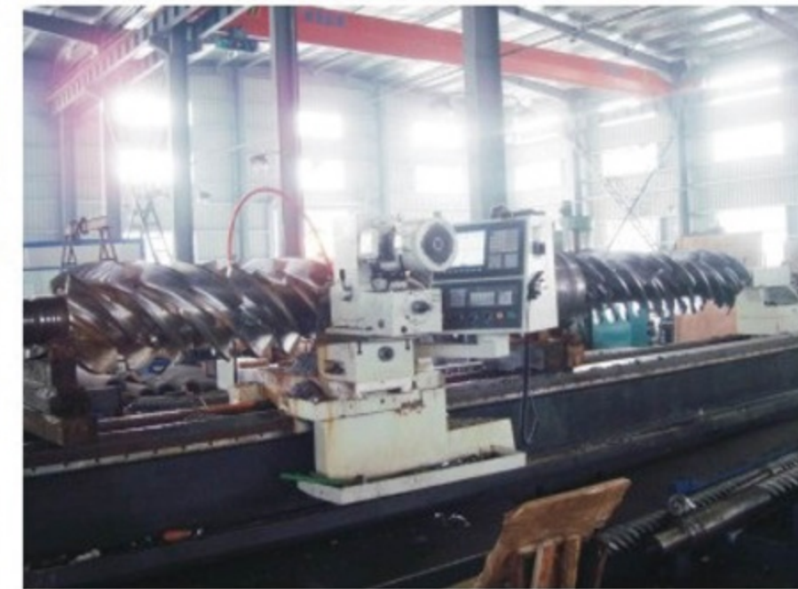
\Phi 500mm \times 10000mm发泡螺杆加工 \Phi 500mm \times 10000mm screw for XPS board in producing
