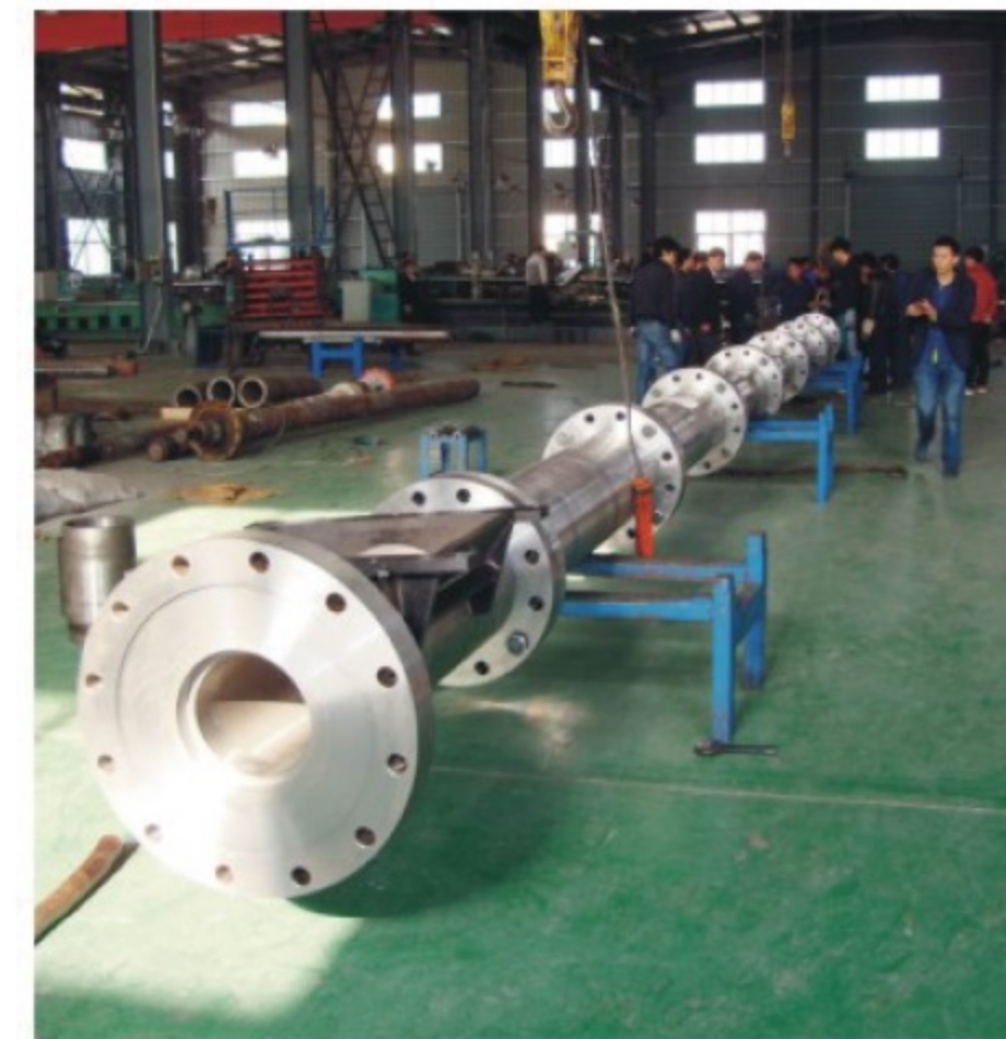
XPS-225机筒螺杆 (孔径Φ250mm, 长15000mm) Φ220 XPS screw and barrel (DiameterΦ250mm, length15000mm)
