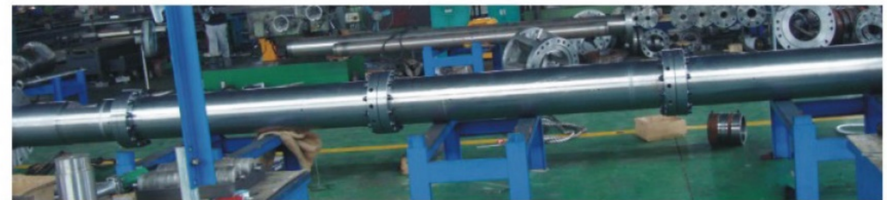
XPS-225机筒螺杆 (孔径Φ250mm, 长15000mm) Φ220 XPS screw and barrel (DiameterΦ250mm, length15000mm)
