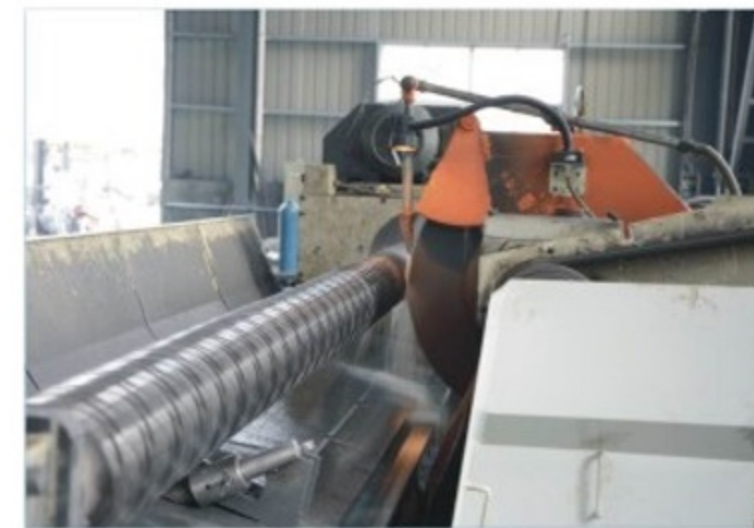
9米大型精密外圆磨床 9 meters ultra-precision cylindrical grinding machine
