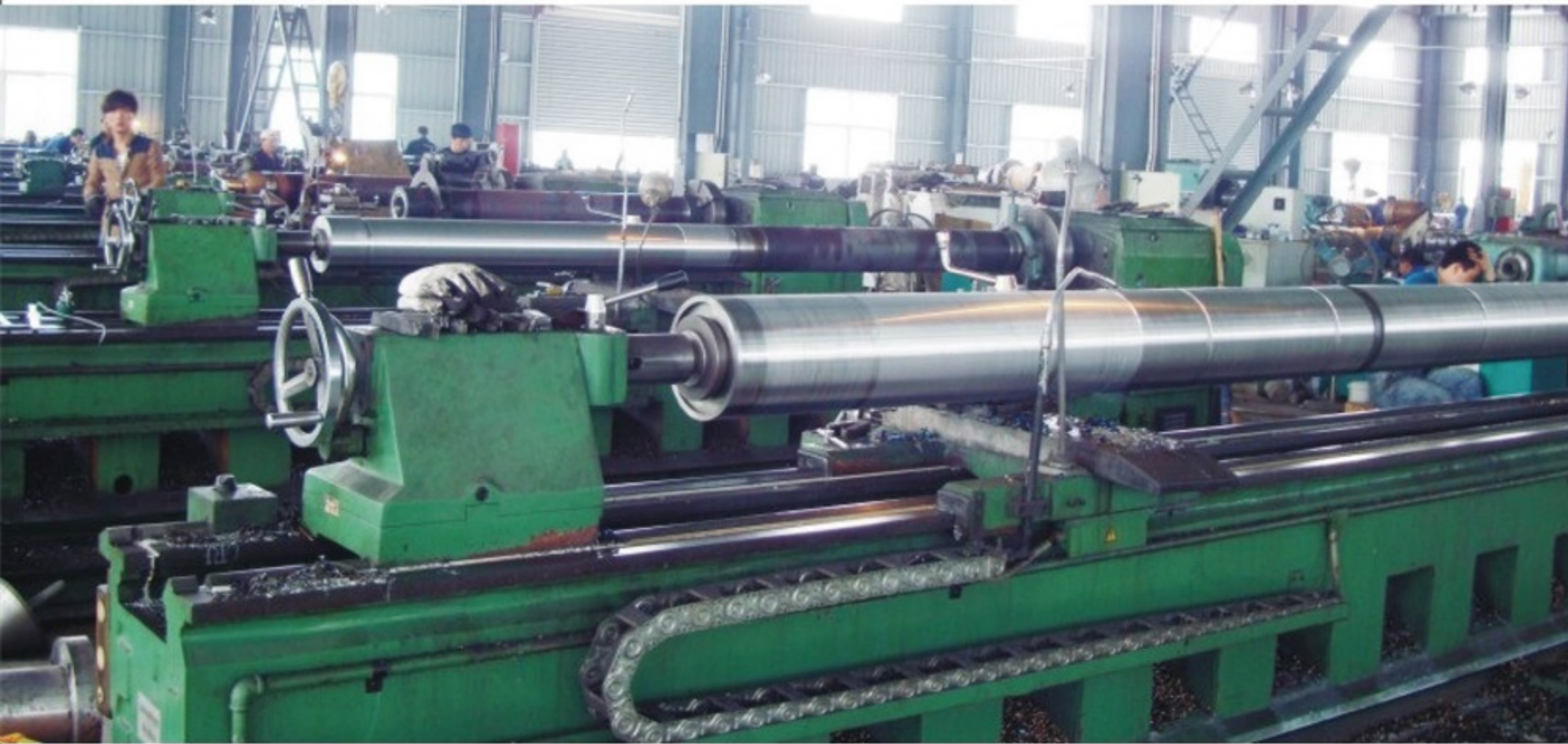
特大型注塑机机筒加工(孔径 \Phi 260mm, 外径 \Phi 1100mm, 长8200mm) The largest barrel for injection moulding machine in producing (Diameter \Phi 260mm, outer diameter \Phi 1100mm, length 8200mm)
