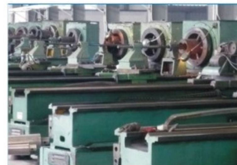
正在加工双孔机筒 Twin barrel in producing
