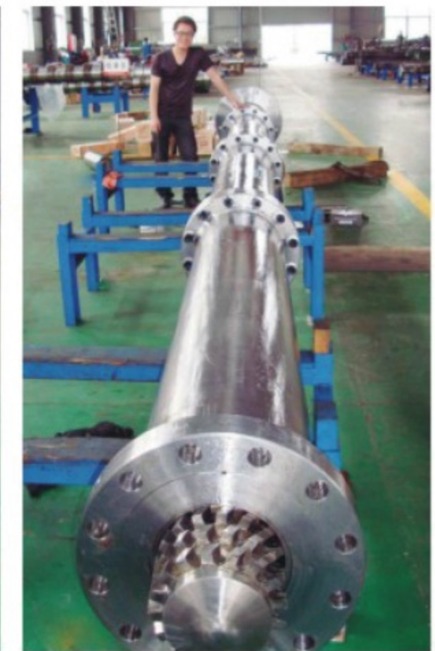
XPS-250二氧化碳发泡机筒螺杆 Φ250 XPS Nitrogen dioxide foam screw and barrel
