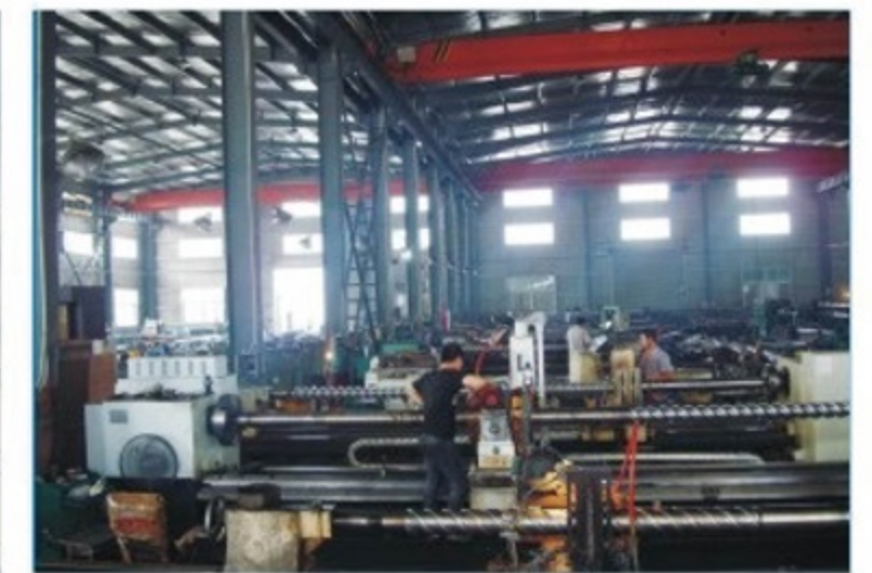
数控螺杆铣正在加工螺杆 CNC screw milling machine in producing
