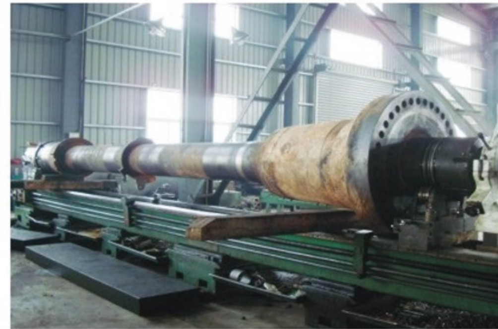
特大型注塑机机筒加工(孔径 \Phi 260mm, 外径 \Phi 1100mm, 长8200mm) The largest barrel for injection moulding machine in producing (Diameter \Phi 260mm, outer diameter \Phi 1100mm, length 8200mm)
